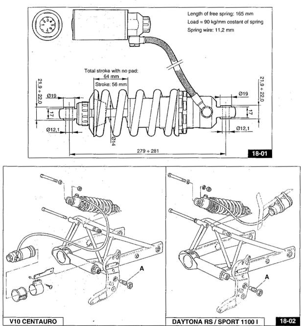
Adjusting the swing arm play (Fig. 18-02 / 18-03) Ensure the swing fork oscillates freely without any play.
