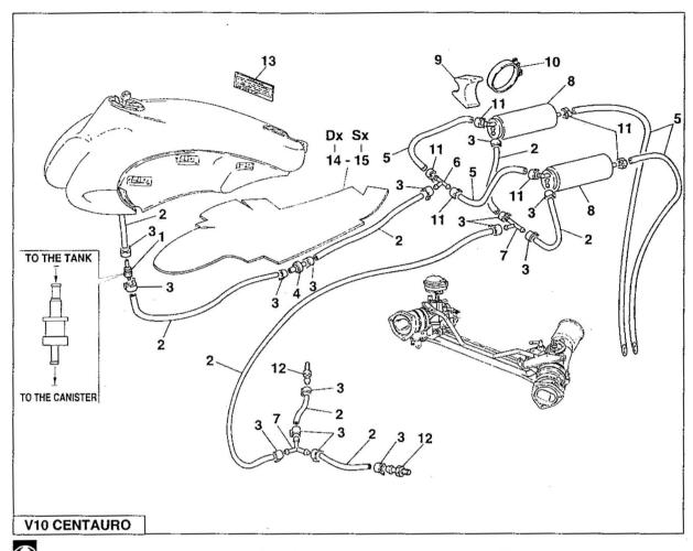
$\bigcirc$  NOTE: The anti-overturning valve Ref. «1» should be vertically installed at ± 30° as regards the exhaust gas inlet located as shown in figure.
