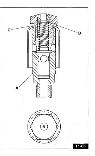
THERMOSTATIC VALVE (Fig.11-89) The thermostatic valve opens the oil passage to the radiator when the temperature exceeds 71°c.
