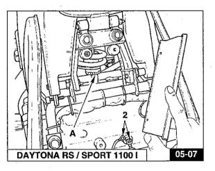
In the V10 CENTAURO model, the adjustment ring nut **«A» - Fig. 05-07** can be reached by removing the saddle (see Removing the saddle in Chapter 3.20) and moving the battery.
