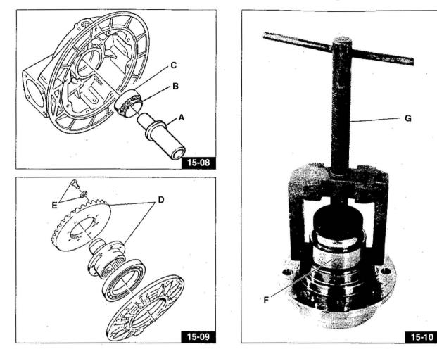
Disassemble the conical pinion support unit.
