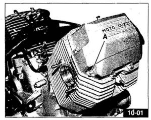
Turn the crankshaft to the T.D.C. position at the combustion stroke (valves closed) of the L.H. cylinder Fig. 10-02.
