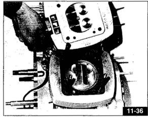
Before replacing the rocker arm support frame, fit the 4 OR rings on the tie rods as indicated in the Fig. 11-37.
