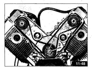
After placing the engine in the TDC position, in the left cylinder combustion phase, check that reference «1»-Fig. 11-48 on the service shaft is lined up with reference «2» - Fig. 11-48 on the timing cover.
