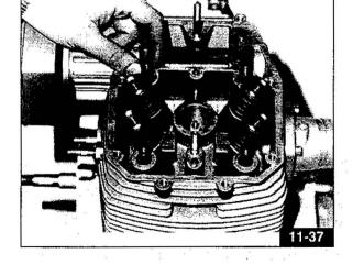
Fit the frame and lock the 4 nuts (dia.10x1.5) to the torque of 4.2÷4.5 kgm in a cross-over sequence and subsequently the two nuts (dia. 8x1.25) at the torque of 2.2÷2.3 kgm (Fig. 11-38).
