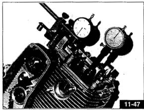
With the engine without the rocker arms, fit a feeler gauge on the left (Induction Control ducket) cylinder discharge command points using the tool cod. 69 90 78 50 as indicated in the Fig. 11-47. The upper timing command pulleys must be without the inner drive gears as indicated in the Fig. 11-47. The drive belts must be stretched correctly.
