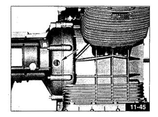
For a more accurate determination of the TDC it is however necessary to proceed as follows: place a feeler gauge with support cod. 30 94 82 00 in the spark plug hole of the left cylinder **Fig. 11-46** and position the piston at TDC. Fit the graduated disk cod. 19 92 96 00 on the crankshaft with hub cod. 30 94 96 00 and relative index cod. 17 94 75 60.
