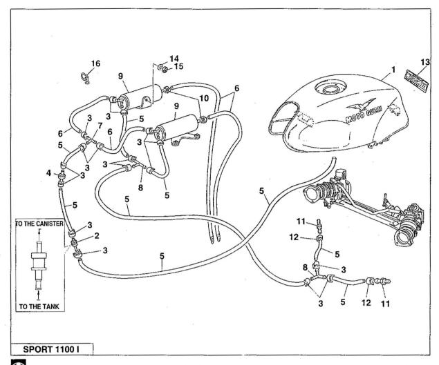
**NOTE:** The anti-overturning valve Ref. «2» should be vertically installed at  $\pm$  30° as regards the exhaust gas inlet located as shown in figure.
