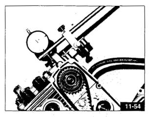
With the graduated disk zeroed with respect to the «A» index and the engine in the TDC position (combustion phase) of the left cylinder, fit a second index «B» in the position shown in Fig. 11-55 (90° from «A» index). Turn the crankshaft in a clockwise direction by 270°; this gives the TDC position (combustion phase) of the right cylinder, with the graduated disk zeroed with respect to the «B» - Fig. 11-56 index.
