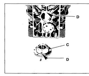
After having assembled the motor shaft in the base, lock the caps coupling screws at Kgm 8,5  $\div$  9,3 torque.
