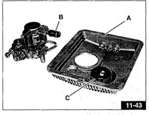
Before mounting the oil sump carefully position the gasket «A» - Fig. 11-43.
