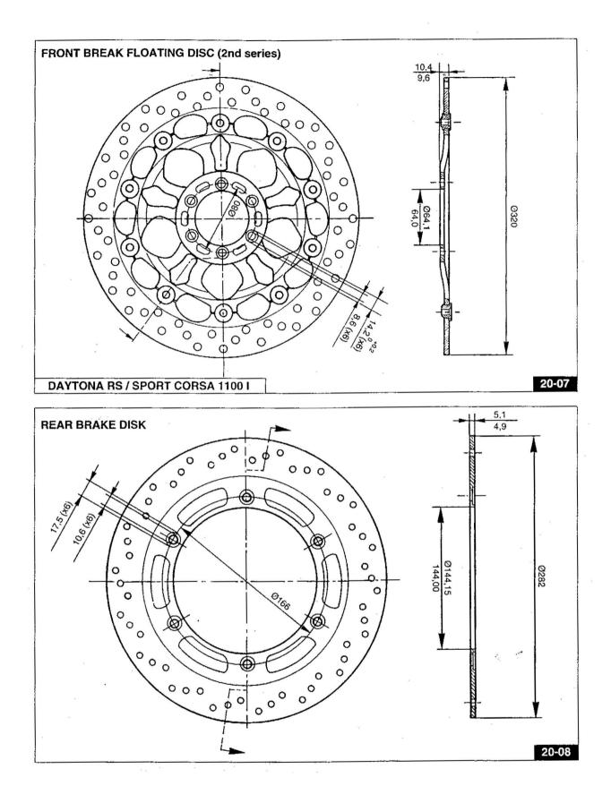
If the rear brake disk has been revised or replaced the "wobbling" should be checked; this check can be carried out by means of a dial gauge and the maximum value should not exceed 0.2 mm.
