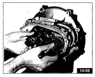
Loosen the internal clutch casing locking ring nut, using the supplied wrenches **«A» - Fig. 14-10**, code 30 91 28 10 and **«B» - Fig. 14-10**, code 14 91 26 03 and remove the internal clutch casing using, if necessary, a universal extractor.
