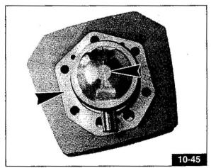
Cylinder and piston should be matched from the same selection marked with a letter stamped on each of them (A with A, B with B, C with C) Fig. 10-45.  Before refitting the rocker arms mount, slip the 4 oil seals «A» into their seats on the stud bolts (Fig. 10-46).
