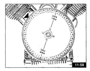
Subsequently check the right cylinder timing as already indicated for the left cylinder and complete the reassembling of the engine unit (Fig. 11-59 / 11-60).
