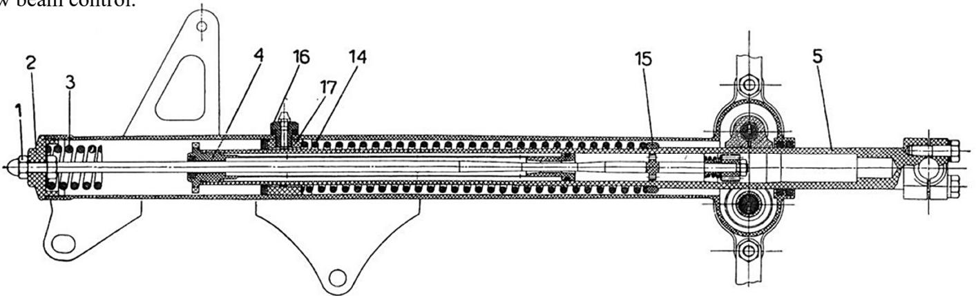
Figure 32- Internals of the telescopic fork.
