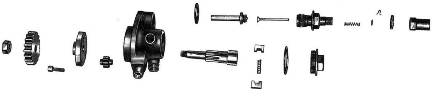
Figure 25- Oil pump dismantled: one notices the sequence of dismantlement.
