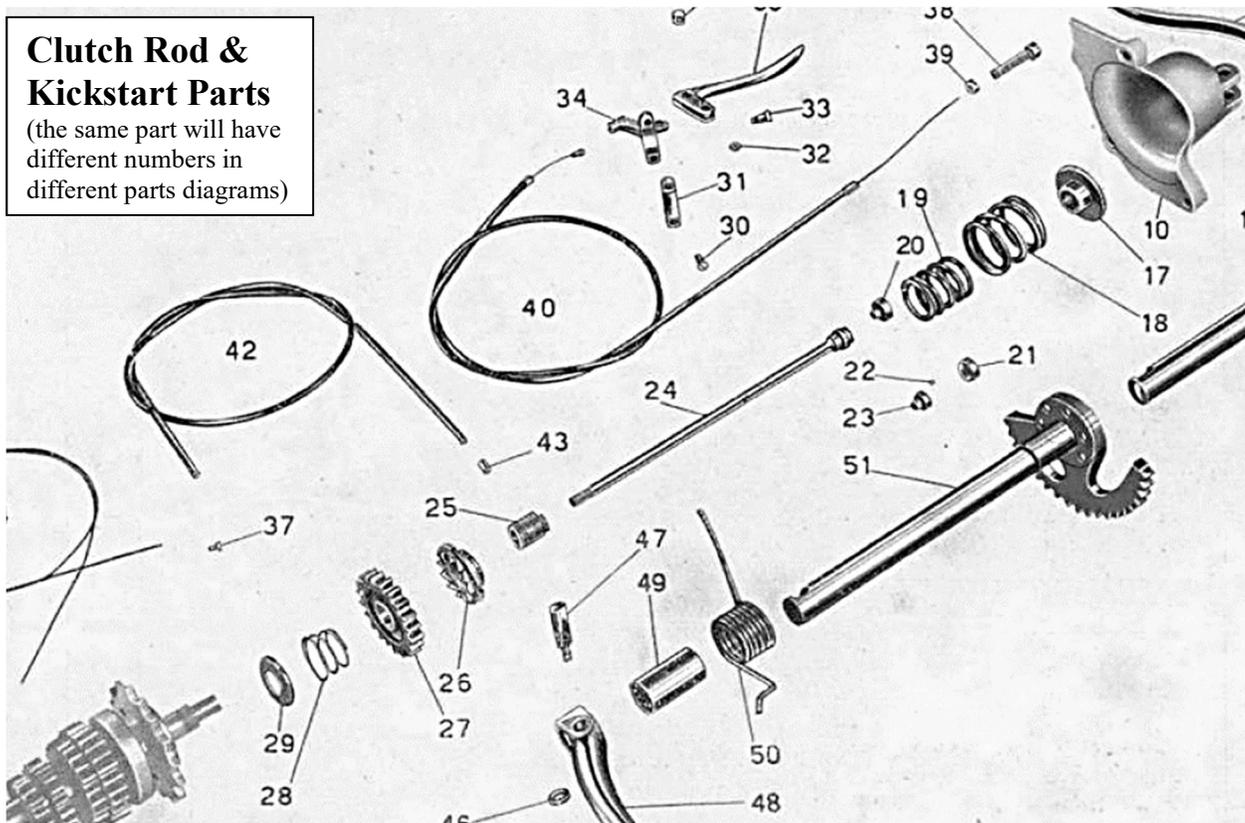
[Under clutch cover] Unscrew the knurled disk [#17 in Clutch Rod parts diagram] with a left-handed thread which pre-loads the 2 concentric clutch springs [# 18 & 19]. Remove the two springs and the internal control rod [#24]. Unscrew it completely by means of flat wrench (view figure 12). Because this can rotate, you need to push the threaded sleeve against the toothed sleeve of the kick starter.
