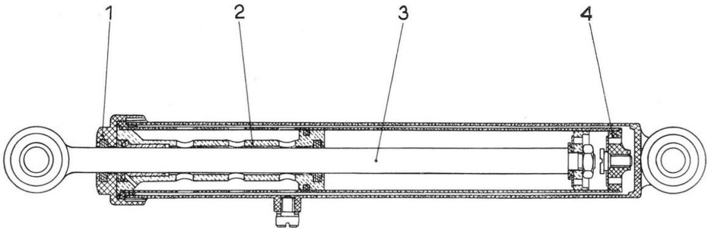
Figure 33- Internals of the rear dampers.
