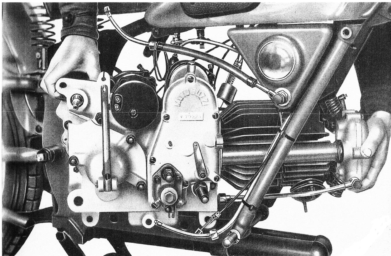
**Fig. 10 – Removing the engine from the frame.**
