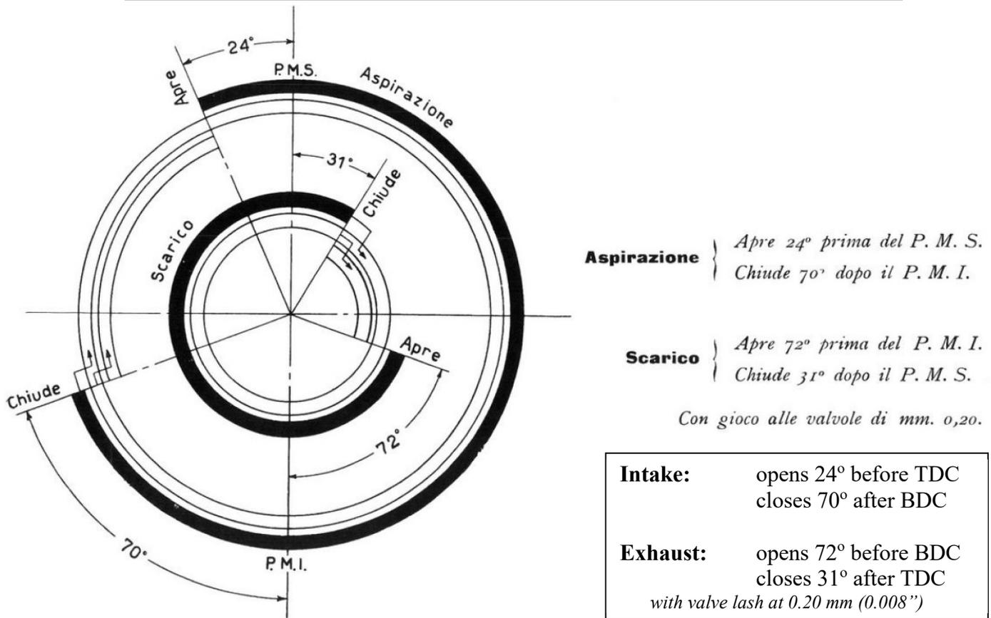
Figure 29- Angular diagram of valve timing related the crankshaft.
