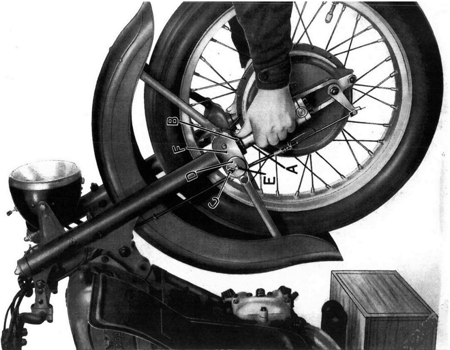
Figure 35- Adjustment of the telescopic fork.
