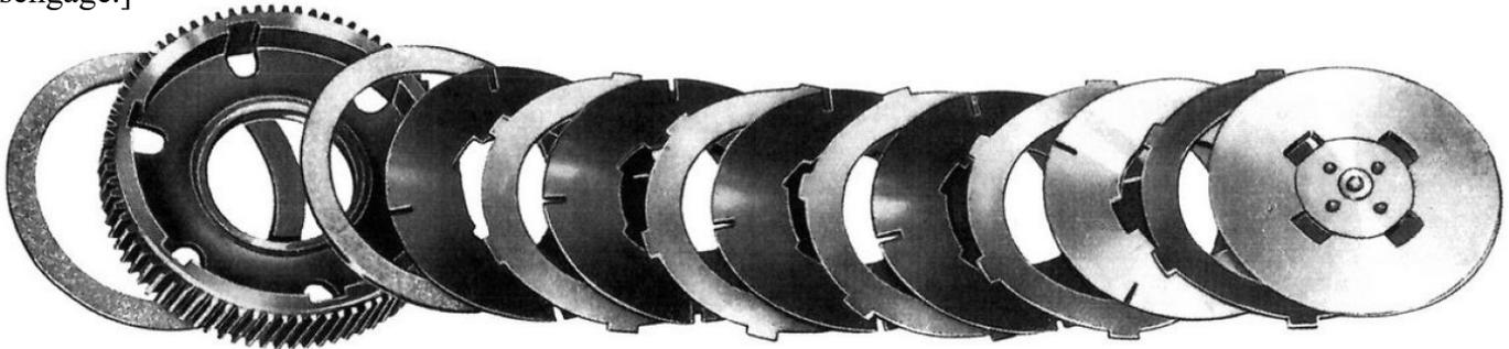
Figure 21- Dismantled clutch (notice the order of assemblage of the varied pieces).
