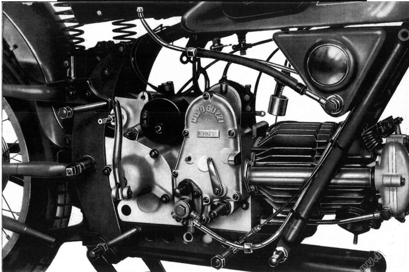
**Fig. 9 – Engine ready to remove from frame. Notice 3 engine fixing pins partially pulled out.**
