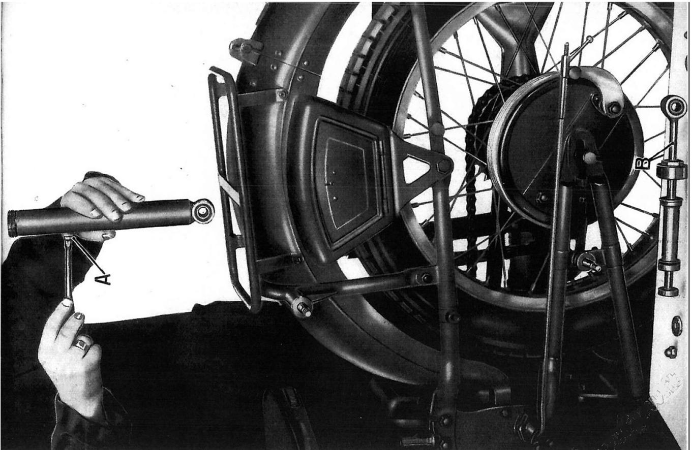
Figure 36- Verification of the liquid in the dampers.
