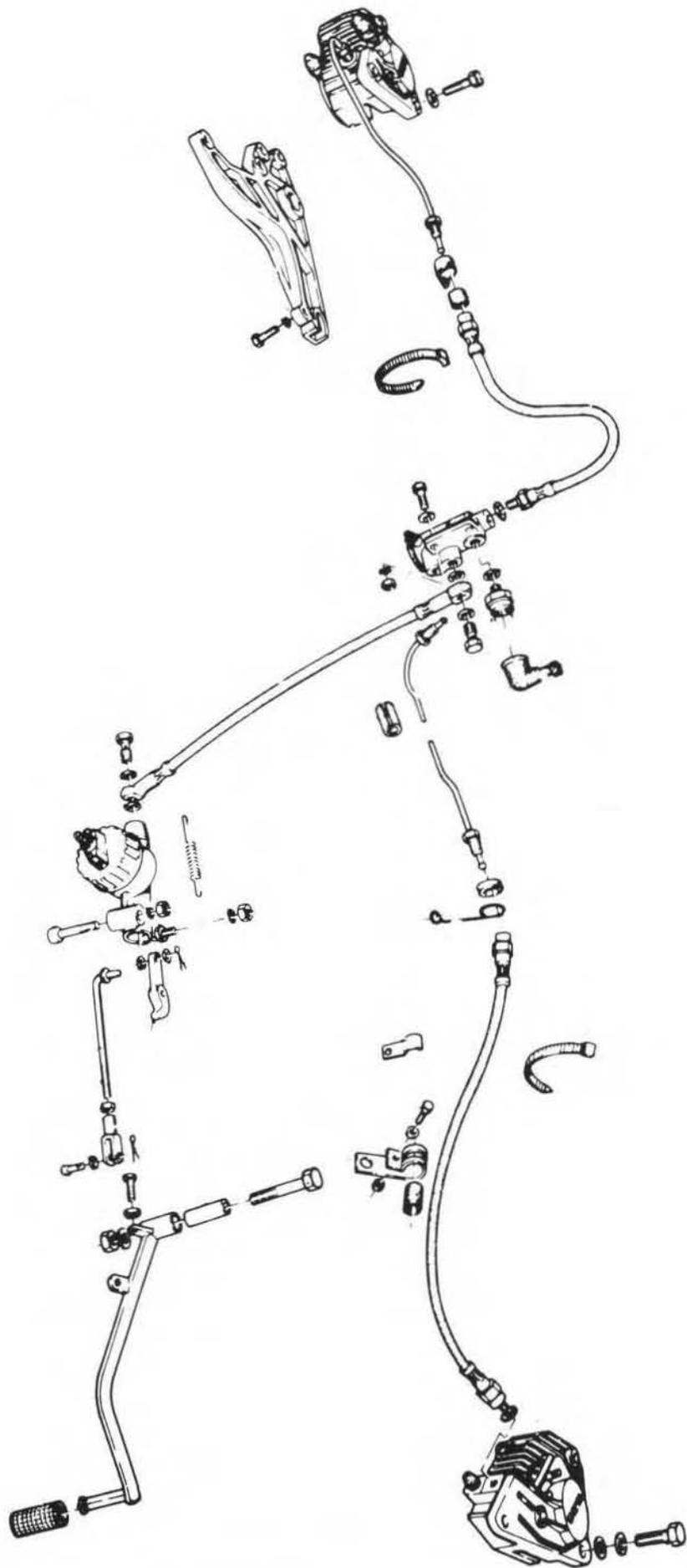
«F» of caliper «E» on the L/H swing fork arm fit transparent flexible pipe «G» with the other end immersed in transparent container «H» partially filled with fluid of same type.
