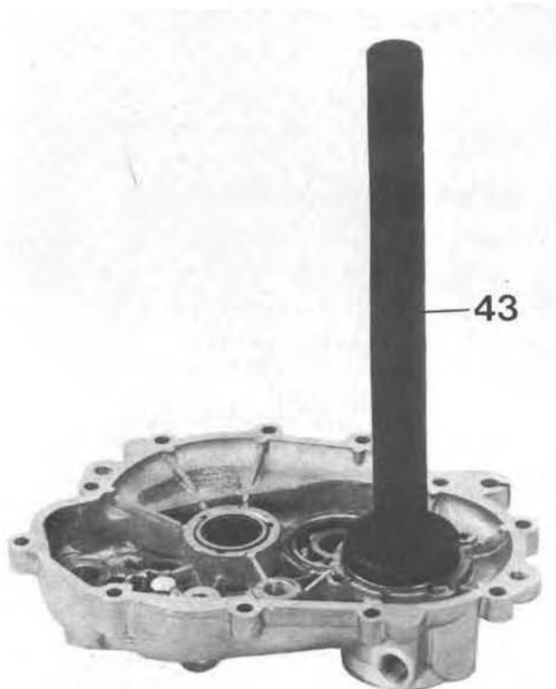
The seal on the gearbox cover for layshaft is fitted using punch N. 14 92 95 00 (48 in fig. 111).
