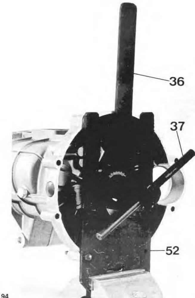
**Removing the gearbox cover components and the selector assembly**
