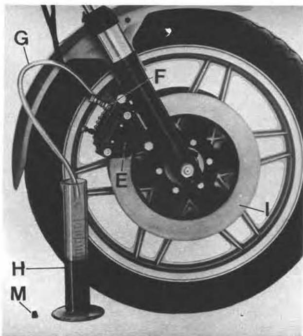
care to avoid possible damages. After cleaning dry up all parts with a clean cloth and lightly smear the cylinder walls and piston with brake fluid to avoid corrosion.
