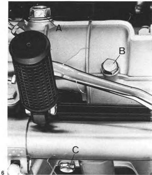
on a warm engine as in such condition the oil is fluid and more easy to drain. Do not forget to let the old oil drain fully before any fresh one is introduced.
