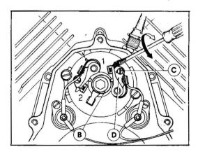
start separating, it is advisable to use an appropriate timing light to be set up between the breaker feeding clamp being checked and the ground.
