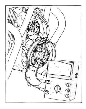
If contact breaker n. 2 does not open in the fixed advance position spamped on the flywheel, it will be necessary to change the contact gap of this breaker, or of both breakers, within the indicated gap of 0.35-0.45 mm.
