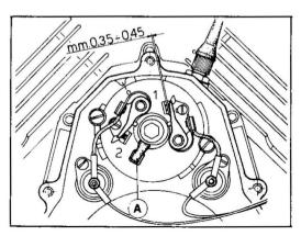
When adjusting the contact points it is necessary to check the ignition timing as well.
