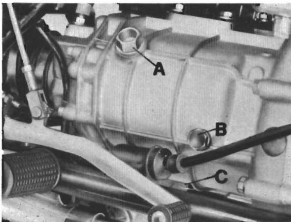
**36** This operation should be carried out a short time after a ride when the oil is still warm and easily drained.
