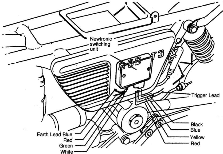
NEWTRONIC SWITCHING UNIT IN L.H. SIDE PANEL
