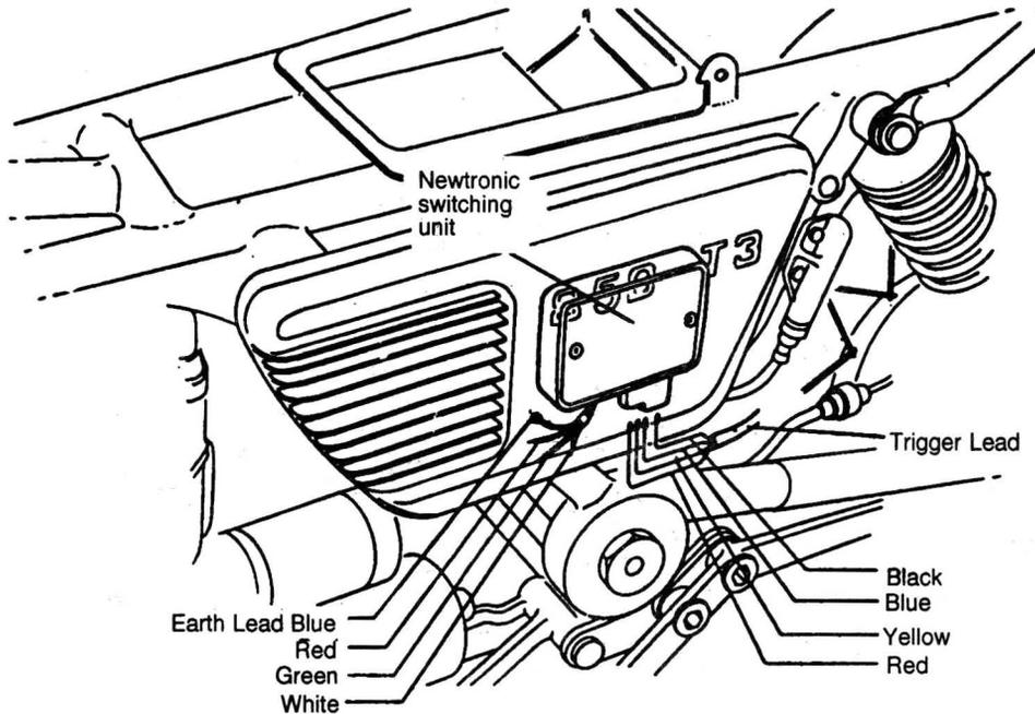
NEWTRONIC SWITCHING UNIT IN L.H. SIDE PANEL
