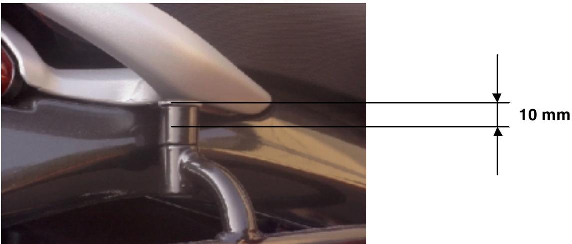
Should this minimum distance of 15 mm not be complied with, the bags could be damaged due to the heat produced by the exhaust fumes.
