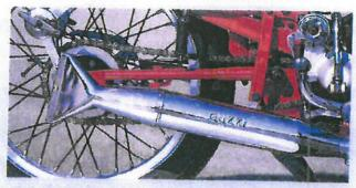
**Exhaust System** - Up to 1956 the typical chromed fishtail silencer with a removable end for cleaning was used. But because of the noise, they were forced to abolish it in favour of a non open-able cylindrical type that, in effect, silenced more but' at the same time, took away a little of the sound and power of the Mandello monocylinder. The front pipe of the exhaust normally tends to become coloured by the heat.
