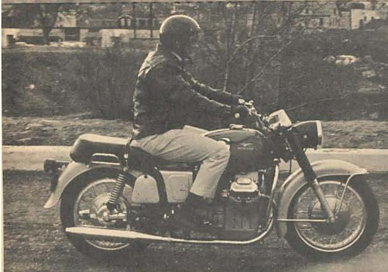
*Some running shots of the big V-7 show that despite its size, it is a smooth-handling machine. And, though it looks massive, the 704cc V-twin actually is lighter than many other tourers. At the bottom left is shown the twin-leading shoe, full width front brake, a good grabber.*
