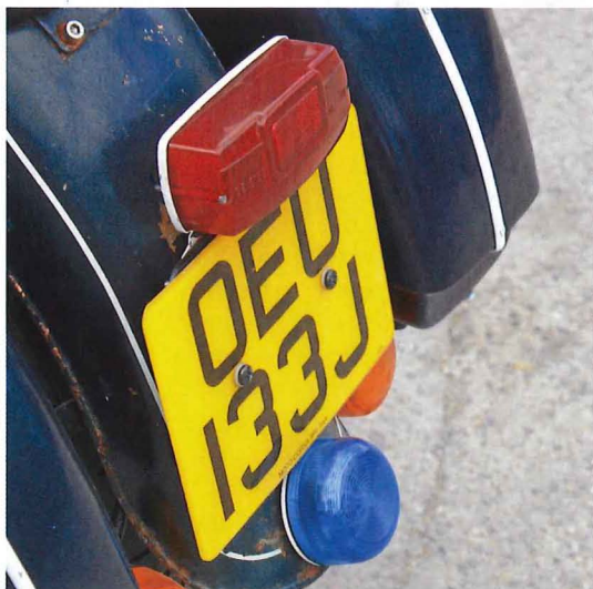
Left: Correct rear light and blue strobe flasher; indicators are probable later addition. 'J' suffix (1971-72) relates to dating certificate.
