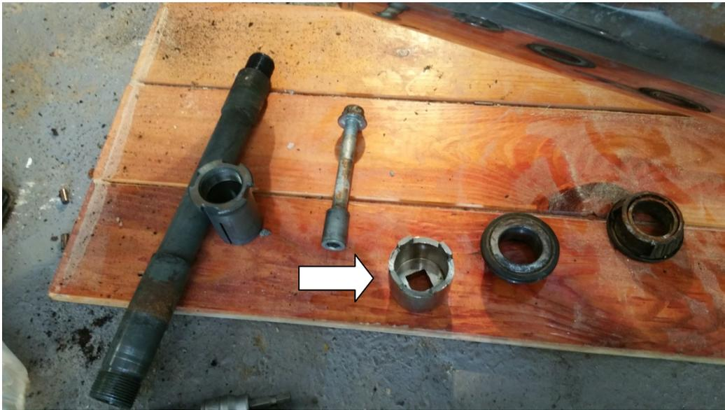
Unscrew the pivot using a 14mm hex. Support the swinging arm and work out the pivot. Mine was rusted and pitted.
