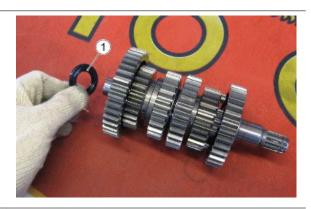
• Remove the gear of the first gear (2)
