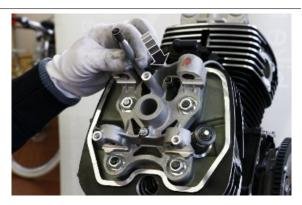
Place the rocker in its seat by inserting the Belleville spring at the same time
