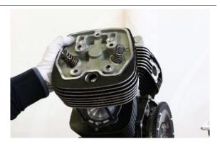
• Remove the cylinder head gasket
