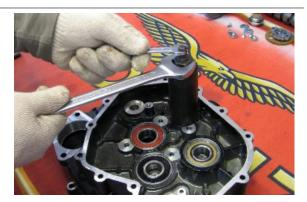
Remove the drive shaft secondary oil gaiter
