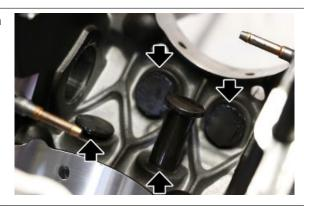
Operating with the engine turned, insert the camshaft in the crankcase paying attention that one of the holes of the small ends matches with the hole with transmitter joint
