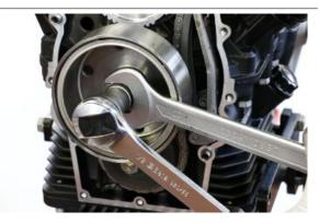
Insert in the rotor hole the specific spacer
