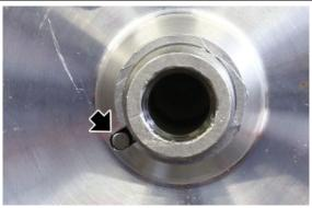
Tighten the three fastener screws of the tone wheel to the specified torque
