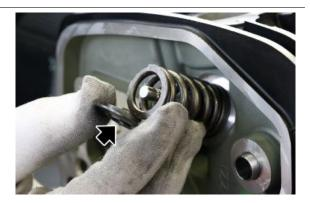
Remove the spring and replace it if it is out of the wear limit.
