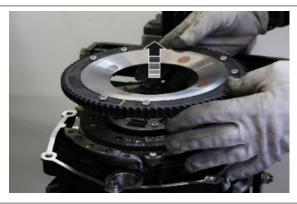
• Remove the clutch plate.
