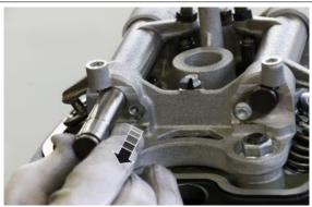
Remove the rocker, being careful to recover the Belleville spring
