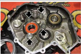
The bearings from the gearbox crankcases can be removed using generic extractors.
