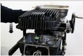
Insert and tighten the 14 fastening screws of the oil sump to the prescribed torque
