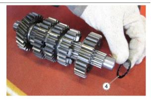
• Remove the gear of the 6th gear (5)
