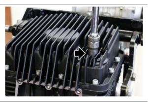
• Remove the engine oil filter
