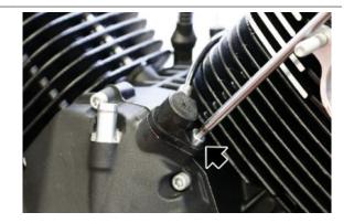
Remove the timing system cover sensor
