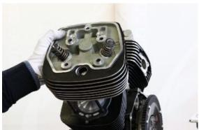
Place the three rubber O-Rings, particularly apply grease to the O-Ring that will be inserted in the stud bolt in order to avoid damaging it
