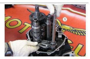
Remove the spring from the index lever
