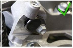
Insert and tighten the fixing screw of the rocker pin lock fork to the prescribed torque
