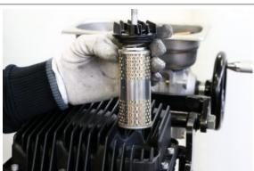
Insert and tighten the locking screw of the engine oil filter to the prescribed torque
