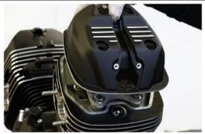
Place the cover fixing screws and tighten them to the prescribed torque
