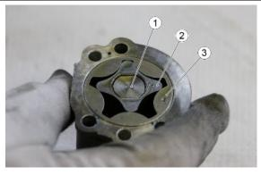
Fit the oil pump in its seat, insert and tighten the three fixing screws to the specified torque
