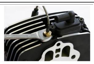
Undo and remove the secondary air valve cover
