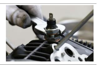
• Remove the transmitter joint
