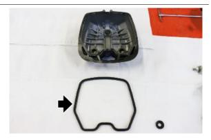
Place the head cover together with the gaskets on the seats of the fixing screws
