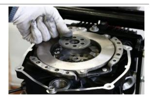
Insert the 6 fastening screws complete with washers and tighten to the prescribed torque
