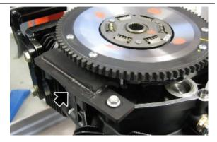
Remove the 6 fixing screws of the clutch plate complete with starter sprocket
