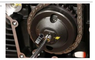
Fit the knurled washer and after placing the nut, tighten it to the prescribed torque
