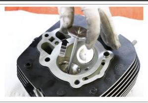
Remove the gasket of the valve guide
