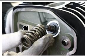
• Remove the valve from the head
