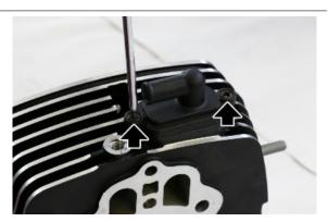
Fit the engine oil pressure sensor, only in the left head and tighten it to the prescribed torque
