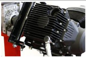
Insert the engine oil filter together with the cover
