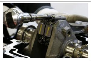
Remove the half-bearings from connecting rods and small ends.
