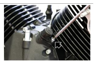
Remove the timing system cover sensor
