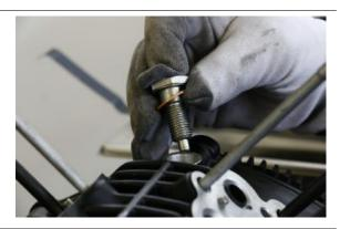
Insert the small ends timing system side and flywheel side on the upper crankcase paying attention to lubricate them
