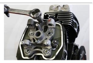
Undo and remove the fastening nuts of the cam tower
