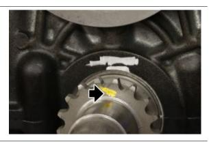
Fit the timing chain together with timing system gear and oil pump gear
