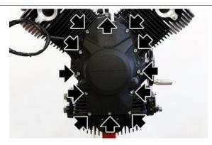
Remove the alternator cover and the gasket
