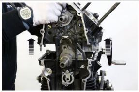
Remove the crankshaft together with connecting rods and small ends
