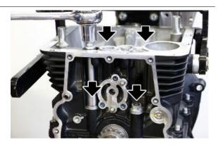
Remove the upper crankcase being careful not to damage its mating face
