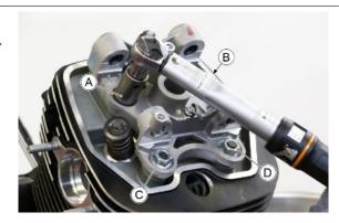
Insert and tighten the compensation nut of the cam tower to the prescribed torque
