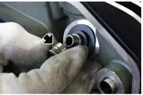
• Remove the lower cap of the spring
