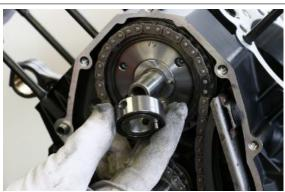
Check and if necessary replace the rubber O-Ring
