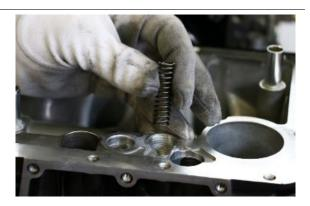
• Remove the overpressure valve
