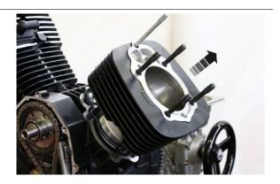
Remove the gasket from the stud bolts
