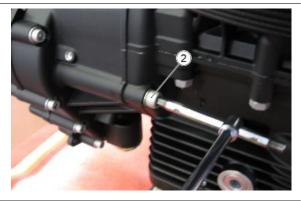
Remove the complete gearbox screw
