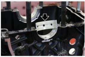
• With the help of grease, place the thrusts on the upper crankcase from the flywheel side, paying attention to lubricate them in the friction area
