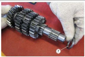
• Remove the gear of the 3-4th gear (8)
