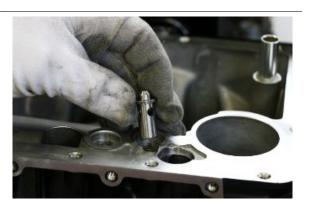
Insert the spring and afterwards the cap provided with a new copper gasket, tighten it to the prescribed torque
