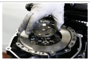
Lock the thrust plate using the special lock ring
