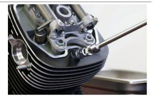
Remove the fastening screw of the rocker pin retainer fork
