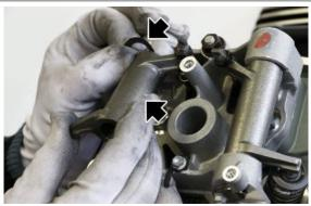
• Using the rocker shim centring pin, align the rocker and the Belleville spring with the pin seat for easy insertion
