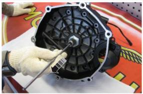
Remove the neutral sensor and take the gasket washer
