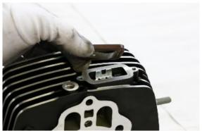
Fit the cover of the secondary air valve and tighten the screws to the prescribed torque
