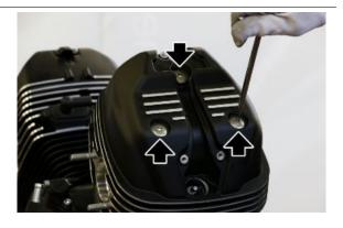
Remove the head cover together with the gaskets
