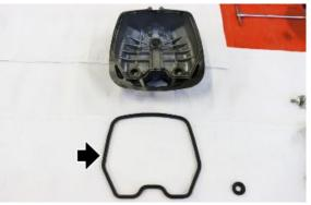
• Check that the mating faces that contact the heads are not damaged or blistered
