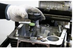
Remove the cap and the relative copper gasket
