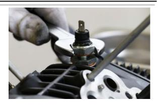
• Remove the transmitter joint
