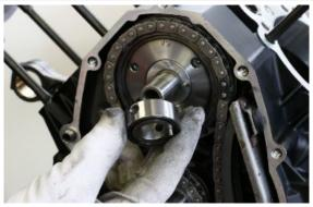
Fit the tone wheel checking the correct positioning on the spacer, using the centring plug
