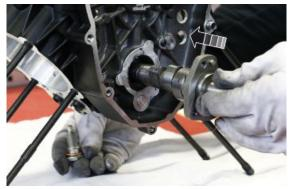
Insert and tighten the transmitter joint to the specified torque
