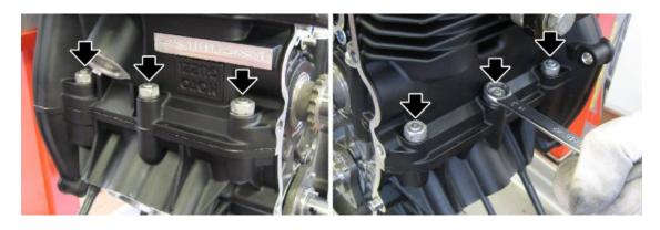
Undo and remove the four long nuts from the inside of the crankcase.
