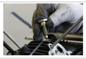
Insert and tighten the oil pressure sensor to the specified torque
