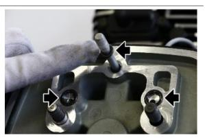
• Position the cam tower in its seat
