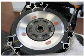
Remove the clutch plate complete with starter sprocket
