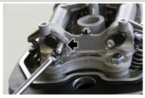
Remove the rocker pin retainer fork
