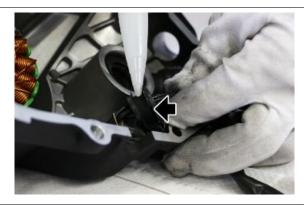
Check that plentiful threebond leaks out and covers all space between the seat on the cover and the cable grommet. Apply another layer of threebond over the cable grommet.
