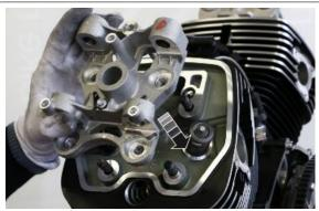
Following a cross order "A-C-B-D" screw the fixing nuts of the cam tower to the prescribed torque
