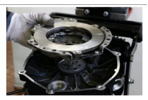
Place the reinforcement flange of the clutch thrust plate, aligning the holes with the ones of the clutch base
