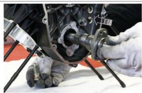
Insert and tighten the transmitter joint to the specified torque
