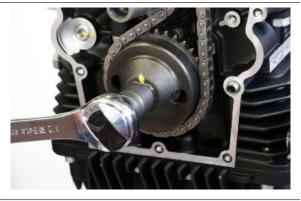
Remove the timing chain, removing the camshaft gear and the oil pump gear at the same time
