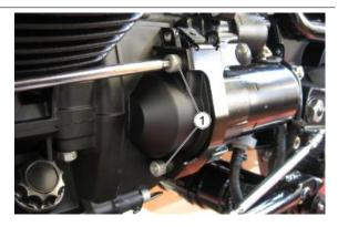
Remove the supporting clamp of the protection (2) and the starter motor (3)
