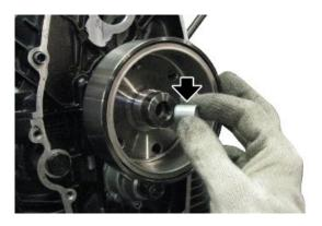
Place the tool (1) on the rotor, tighten the threaded pin (2) of the tool and proceed with the rotor removal
