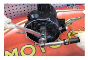
Remove the clutch shaft with a few mallet (1) strokes
