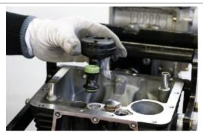
Place the gasket and insert the oil sump cover
