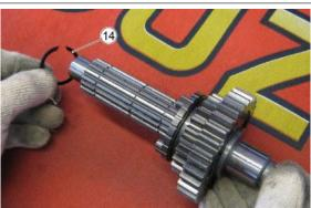
• Remove the gear of the 6th gear (15)
