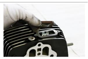
Remove the internal filter paying attention to the direction during refitting
