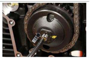
Fit the knurled washer and after placing the nut, tighten it to the prescribed torque
