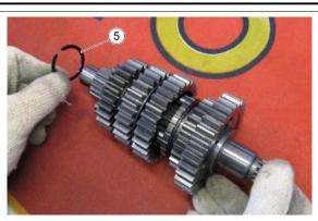
• Remove the gear of the 5th gear (6)
