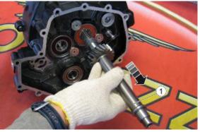
Remove the oil seal from the clutch shaft
