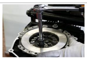
Remove the reinforcement flange of the clutch thrust plate
