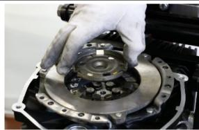
• Remove the 6 fixing screws of the locking plate
