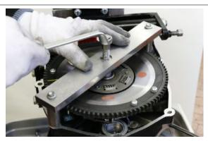
Fit the assembly on the pressure plate flywheel, insert the six fixing screws and tighten them to the prescribed torque
