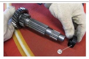
Remove the washer (13) from the main shaft (14)
