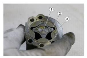
Remove the bearing from the pump body
