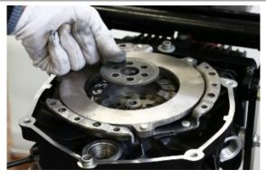
Remove the clutch lock complete
