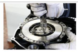
Remove the thrust plate
