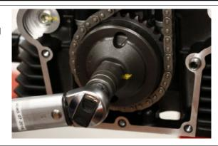
Fit the spacer checking the correct positioning on the blow-by cap, using the centring plug
