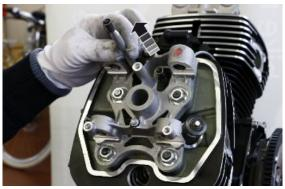
Unscrew and remove the compensation nut of the cam tower
