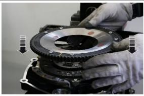
Using the special tool for the centring of the clutch plate
