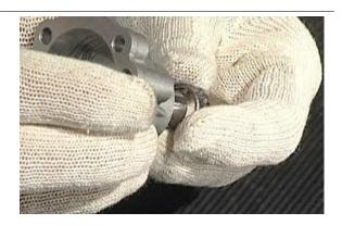
• Insert the external rotor (3), the internal rotor (2) and the pin (1) on the pump body paying attention to match the punching present on the rotors and that both are visible
