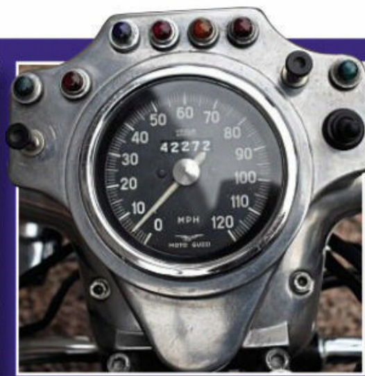
Relics of police service include the remarkable 'dashboard', the curiously situated ignition switch and the painted-over welding 'scar' left by removing the friction horn
