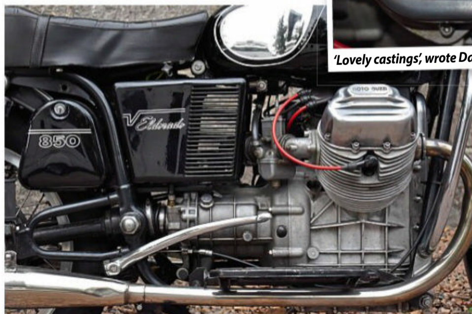
The right side of the engine is as handsome as the other side, but has the driveshaft all to itself
