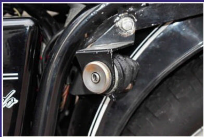
Relics of police service include the remarkable 'dashboard', the curiously situated ignition switch and the painted-over welding 'scar' left by removing the friction horn
