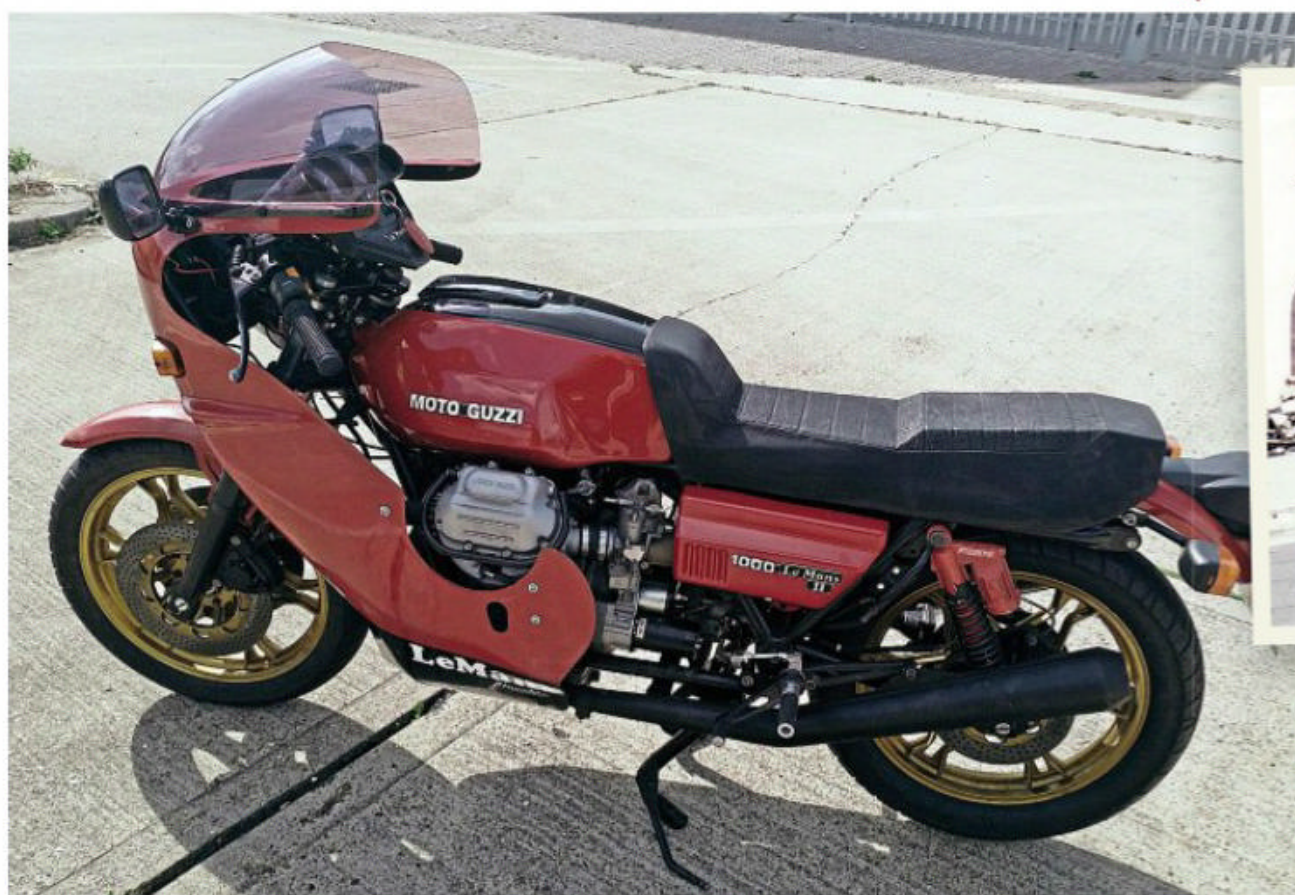
Built by Agostini to DMB's engine spec, this V1000 Le Mans was originally shipped to South Africa with its factory bodywork. Over time it's been modified with a Stucchi fairing, revised rearsets and a new paint scheme
