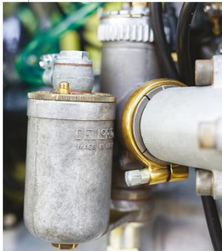
Early V7s used remote float Dell'Orto SS1 carbs (left). Frame and engine numbers weren't factory matched; the engine is number 1337 (top). The valve covers are polished to an other-worldly shine. Motogadget LED bar end signals were added for visibility.
