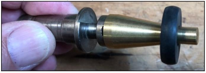
Piston Seal in place after being pushed on using the adapter:
