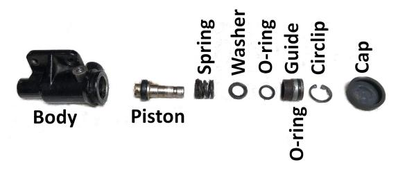
All parts should be cleaned and inspected carefully prior to assembly. All ports in the Body should be clean and clear. Internal bores in the body should be smooth and free of major wear marks.
