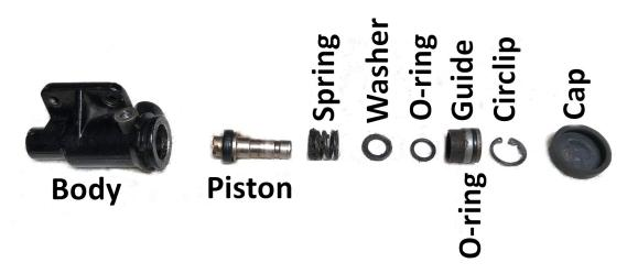
All o-rings and rubber seals MUST be EPDM as they are immersed in DOT4 brake fluid. The Piston Seal was made to order by a local seal supplier.
